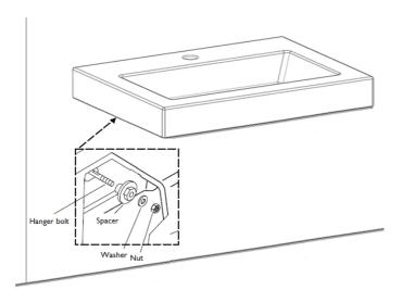
Place the spacer, followed by the washer onto the threaded hangers and then hand tighten with the nut, place a level along the back edge and check before fully fastening.
