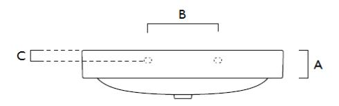
Remove the basin from its packaging, and measure the distance A (Depth of basin) B (width of fixing holes) C (distance between top edge and centre of fixing hole)
