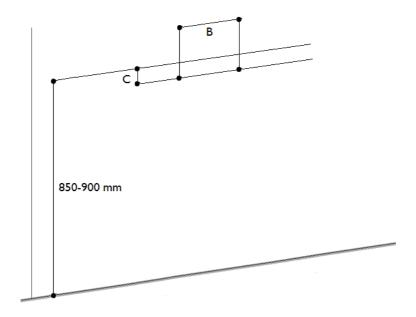
Mark a line horizontal of 850-900mm, this is a recommended height that the wall mounted basin should be installed at, Using the basin measurements mark line C and line B.
