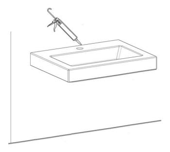
To finish place a small bead of silicon along the back edge of the wash basin.
