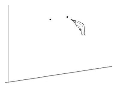
Using the wash basin fixing kit, gauge the correct diameter and depth for the wall plug and use corresponding drill bit to make the holes in the surface.
