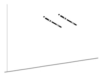
Insert the wall plug, and then screw in the the threaded hanger bolt to the required depth.
