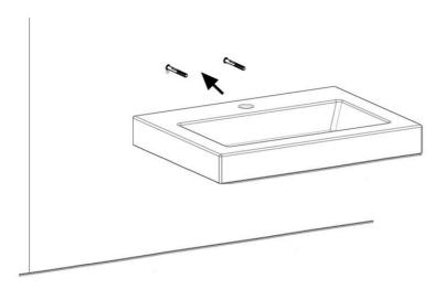
Install the wash basin onto the threaded hangers, a second person will be required to hold the wash basin in position whilst fixing.
