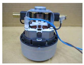
3. Remove and retain both motor rubbers on the top and at the bottom. Place the two motor rubbers on the new motor. Reverse Steps 1 and 2 to place the new motor firmly in the motor housing.
