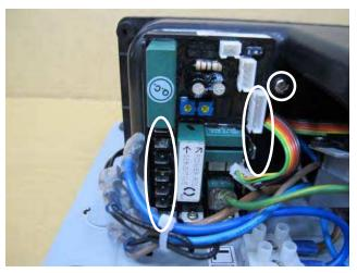
1. Pull off the six wires and remove the fixing screws of the timer.
