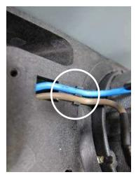
4. To replace the motor, install the motor rubber (large/small) on the motor, and place the motor under the fan blower. The wire set must be fixed to the ditch in the lower housing of the blower.
