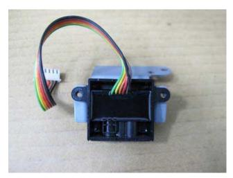
4. Remove the black screws on the senor. Install the new sensor and reverse Steps 1~3 to fasten the sensor.
