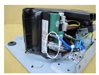
1. Remove the wires that connect heater to the timer.
