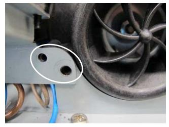
3. Remove the screws from the sensor bracket to take out the sensor.
