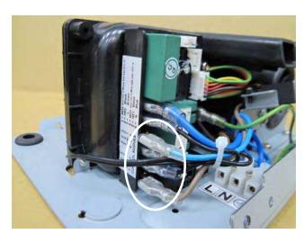
1. Remove the wires that connect motor to the timer.
