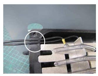
3. To replace the heater, the wire set must be fixed to the ditch in the lower housing of the blower.
