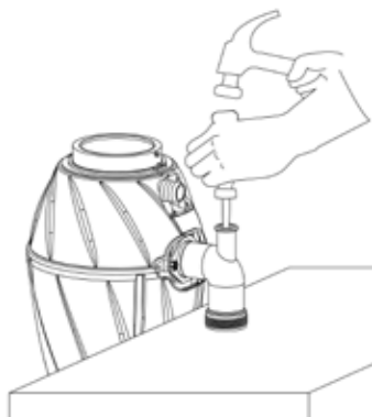
Removal of the diaphragm
