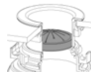
Correct position of the protective gasket
