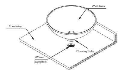
Place the wash basin on the mounting collar and then onto the countertop, take notice of the spout length of the mixer so that the distance to the waste hole is correct. Mark around the inside perimeter of the mounting collar. Drill the waste hole with correctly sized holesaw.
