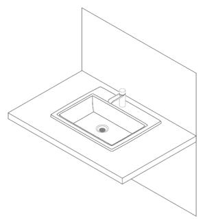
Install the Basin Mixer, Waste and Trap If required run a further small bead of silicon around the perimeter base.
