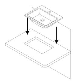
Place the wash basin in position, rempve any excess silicon and allow the silicon to cure for a few hours.
