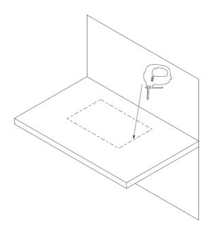
Using a Jig-saw, cut around the mark, after cutting it is advised to seal the bare wood with some PVA (or Similar) sealant.
