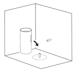
Re-position the basin into the fixing area, connect the waste as per your required waste location(wall drain or floor drain). Before putting the basin into the final position, pour some water into the basin to ensure there are no leaks from the waste.
