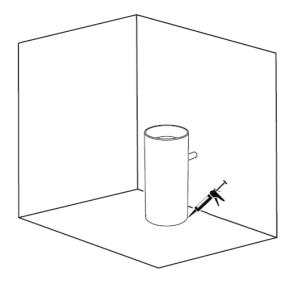
Finalise the position of the basin and run a small bead of silicon around the perimeter base.
