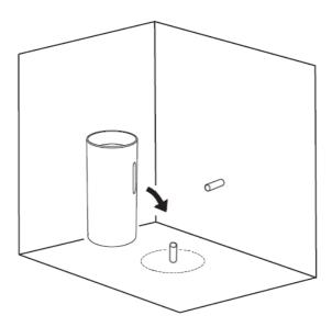
Re-position the basin into the fixing area, connect the waste as per your required waste location(wall drain or floor drain). Before putting the basin into the final position, pour some water into the basin to ensure there are no leaks from the waste.
