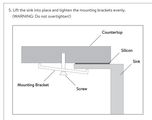
6. Apply a bead of silicon sealant at the edge of the sink fill any gap. Wipe away any excess silicon and allow to dry.
