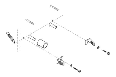
From the vertical line measure the thickness of the semi-pedestal, now draw the horizontal line through from the fixing hole. Offer up the fixing bracket so that the edge aligns with the inner vertical line. Mark the fixing hole, drill plug and bolt the fixing in place.
