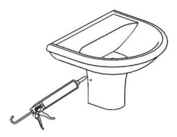
Clean away the pencil lines and if required place a small bead of silicon around the semi-pedestal
