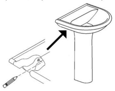
Before removing the basin, from the underside mark the wall anchor points as shown above
