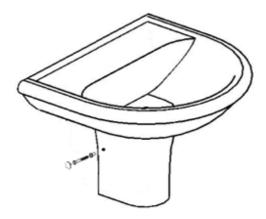
Secure the semi-pedestal to the fixing kit with the plastic sleeves and the screws. Fit the plastic cover caps over the heads of the screws.
