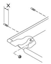
Install the threaded rod fixing into the wall, measure the thickness of the basin ceramic and add 25mm this will give you 'X', ensure X is petruding from the wall to allow fixing.
