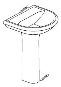
Once level, draw a pencil line around the bottom perimeter of the pedestal and a line across the top edge of the basin, this will give a reference mark when re-installting after drilling.
