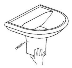
Hold the semi-pedestal in position under the basin, and mark the fixing hole and outer perimeter. Remove the semi-pedestal and remove the basin.
