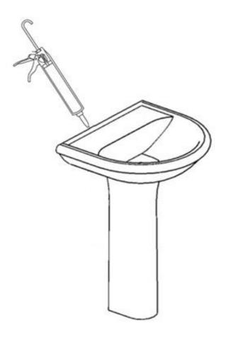
To secure the pedestal, place a bead of silicon around the base perimeter, and if required the joint between the basin and pedestal.
