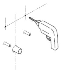
Remove the Basin and pedestal, the anchor point should be clearly marked.
