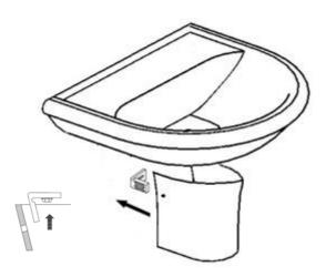
Connect the flexible pipes to the angle valves, Connect the waste and bottle trap to the waste pipe, test for any leaks. Place the semi-pedestal back into position over the fixing kit.
