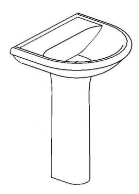
Place the pedestal in position, and place the basin on top, align the 2 items so that items are level. Also check that the basin is sitting flat against the wall.
