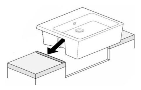
Place the basin in position, make sure to wipe away and excess silicon. Allow to dry.
