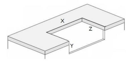
Use the dimension from the basin and mark and cut out the area.
