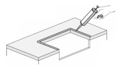
Place a layer of silicon onto the countertop edge.
