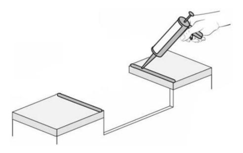
Place a layer of silicon onto the countertop edge.
