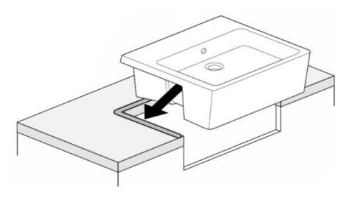
Place the basin in position, make sure to wipe away and excess silicon. Allow to dry.
