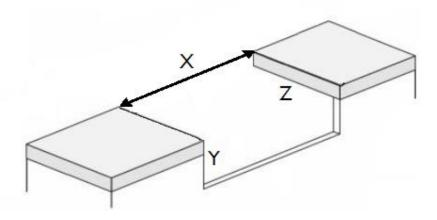
Use the dimension from the basin and mark and cut out the area.
