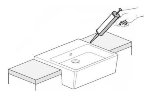
Apply a small bead of silicon around the perimeter of the basin. install Brassware and waste to the wash basin.
