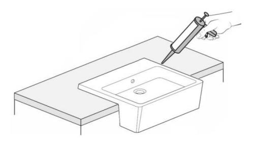
Apply a small bead of silicon around the perimeter of the basin. install Brassware and waste to the wash basin.
