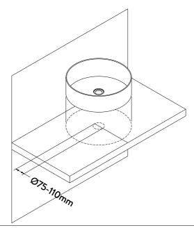
Install the waste assembly into the basin.
