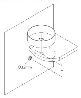
Drill waste hole allowing for the finished dimensions of the waste outlet. In this instance its 75-110 mm, please check your corresponding waste outlet product.
