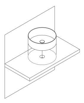
Install the bottle trap onto the waste, cut the horizontal pipe to length and install into the wall via a waste compression fitting or rubber socket.
