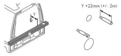
Place a level along the back-side of the bidet, take the measurement to the center of the fixing hole (Y) add 22mm (+/-2mm), Thread the fixing bolt into the desired position and have the grooves pointing outwards, then insert the flush and the waste pipe. Then install the bidet onto the fixing bolts
