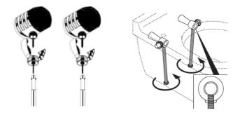
Click the extension rods into the fixing kits, and install the Bidet onto the fixing bolts.
