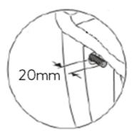
Place the WC onto the fixing bolts, and leave 20mm of thread showing through the ceramic, then insert the flush and the waste pipe.
