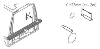
Place a level along the back-side of the bidet, take the measurement to the center of the fixing hole (Y) add 22mm (+/-2mm), Thread the fixing bolt into the desired position and have the grooves pointing downward, then insert the flush and the waste pipe.
