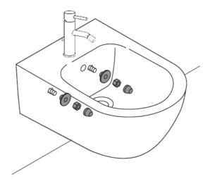
Ensure the bidet is level, then Install the washer and nut and tighten, to complete place the cover cap the over the top of the bolt.
