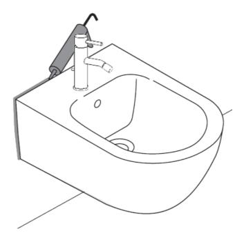
Connect the waste trap, if required place a small bead of silicon around the perimeter of the Bidet.
