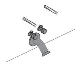
Ensure that the plumbing provisions projecting from the wall are suitable for the bidet installation.
