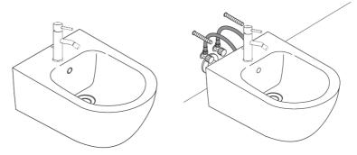
Install the desired bidet mixer and waste outlet to the bidet
